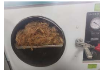
Figure 4. Desiccation process of Banana fiber
