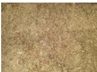
Figure 3. Banana fiber after surface treatment
